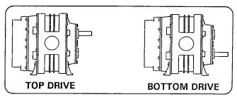
If the unit is horizontal, then the shaft location would be either left or right side.
