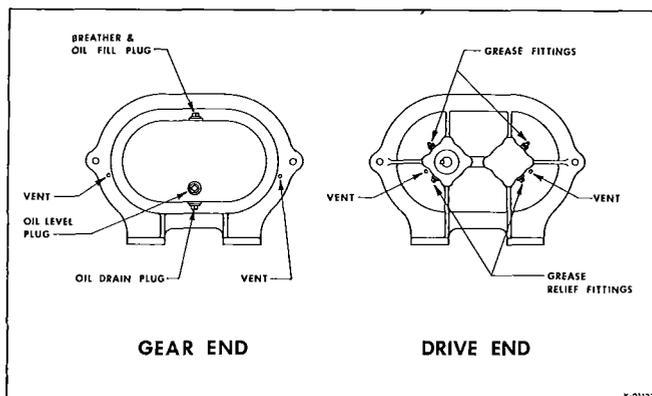
Figure 4 - Lubrication Points
