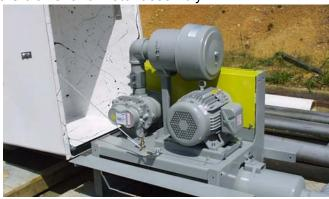
The motor side leg is provided with an indexed slot to mount discharge silencer supporting brackets. The indexed slots take the guess work out of silencer location and ease assembly. Complimen-
