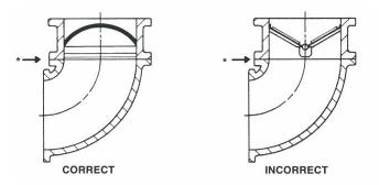
*NOTE:* Frequently the discharge of pumps and compressors simulates the above elbow configuration, which causes higher velocity at the outer circumference. Care should be taken to position values as shown above for these applications.
