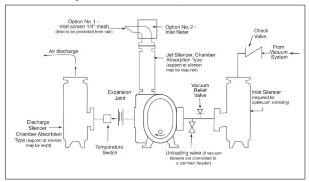
Figure 2 - 700 Series DVJ Air Blower Installation with Accessories
