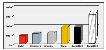
\*Total water content by Karl Fischer analysis during Kaydon testing as defined: based upon a constant initial water ingression of 5000 ppm; test run at 120°F (49°C), 6 gpm.
