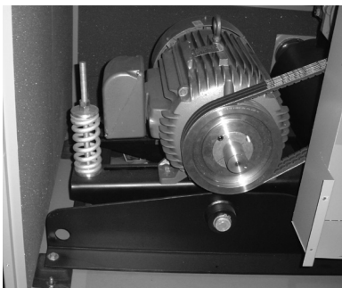
Patent pending, spring loaded automatic v-belt tension system.
