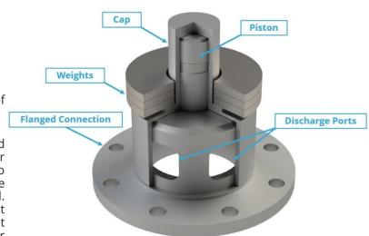
**INSTALLATION**: Install with full face flange only. Relief valves must be mounted in the vertical position to assure proper operation. The relief valve is installed on the discharge side of the blower, before any valves, preferably immediately after a silencer if one is supplied.
