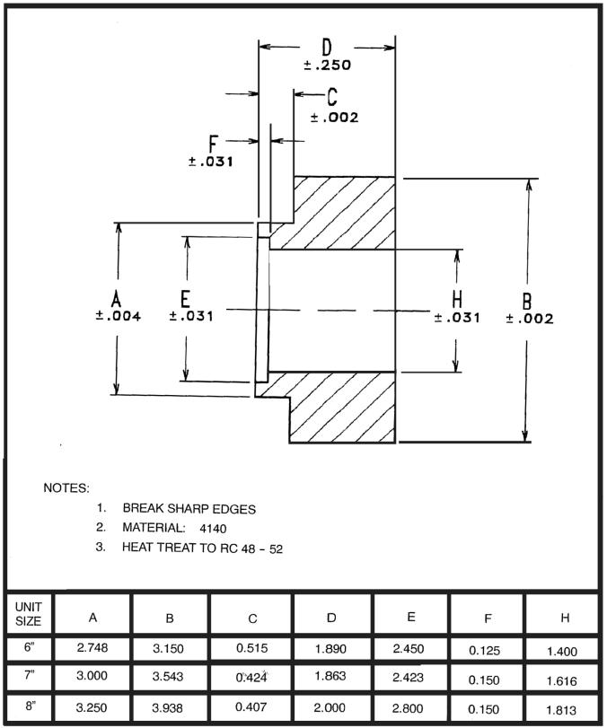
FIGURE 5-3 – MECHANICAL SEAL INSTALLATION TOOL – SK2152
