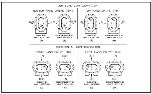
FIGURE 2-1 – BLOWER MOUNTING CONFIGURATIONS
