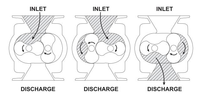
Figure 4-1 – General Operation Principle
