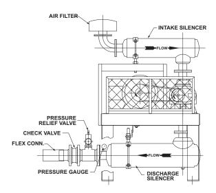
Figure 5-1 – Typical Blower Installation
