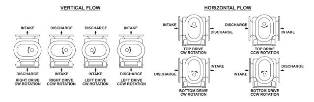
Figure 4-2 – Flow Direction by Rotation
