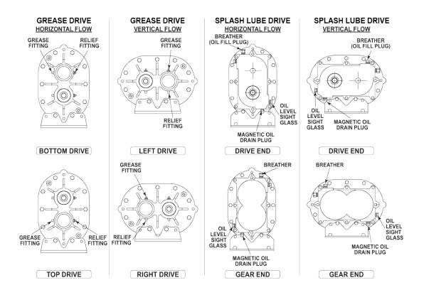
Figure 5-3 – Location of Oil Fill, Drain and Level Gauges on CP Series Blowers
