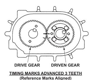
Figure 8-3 – Timing Marks Advanced Three Teeth
