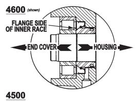
For Model 4500, install bearing so that flange side of inner race faces outward.
