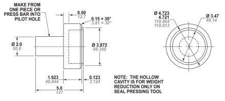
Figure 13-4 – Model 6000 Seal Pressing Tool
