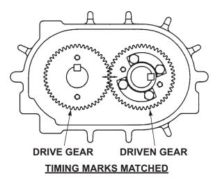
Figure 8-2 – Timing Marks Aligned
