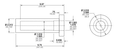
Figure 13-2 – Model 4500/4600 Bearing Installation Tool
