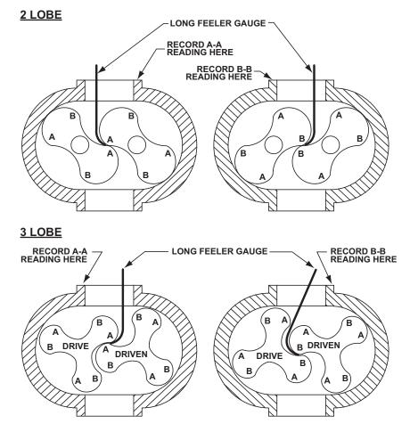
Figure 8-6 – Checking Rotor Interlobe Clearance
