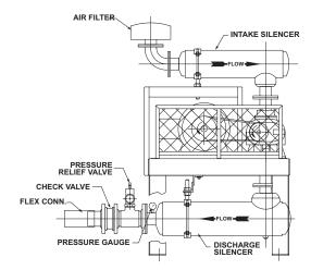
Figure 5-1 – Typical Blower Installation
