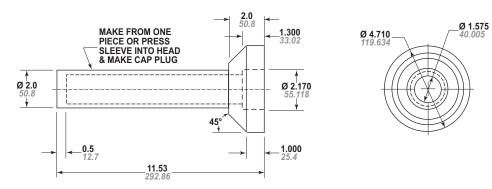
Figure 13-3 – Model 6000 Bearing Pressing Tool
