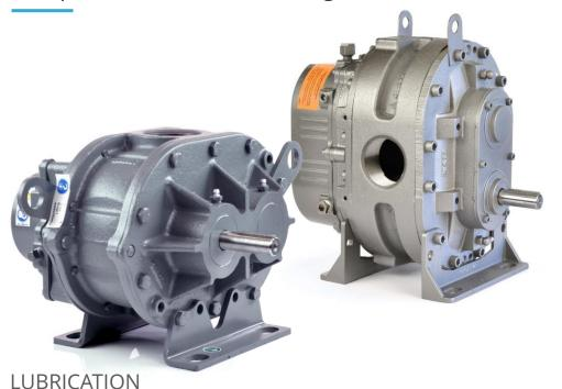
Both the 33 URAI and 3M Legend utilize oil lubrication on the gear end and grease on the drive end.
