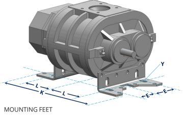
Both the ZZ3L (pictured above) and 36 URAI (pictured left) have oval mounting slots in the feet. If switching to a ZZ3L, check dimension K as the feet extend further out and could conflict with other items in a blower package such as drive guards.
