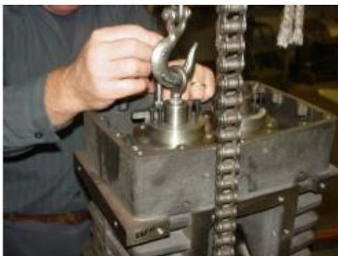
**FIGURE 8-2 – MEASURE STEP IN FALSE BEARING**
