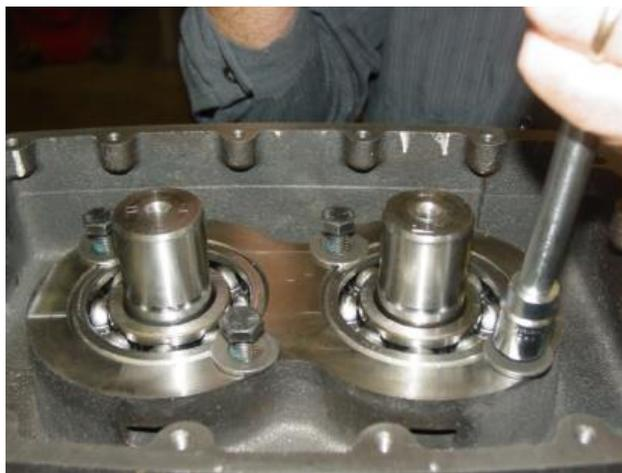
**FIGURE 8-4 – INSTALL BEARING RETAINING SCREWS**
