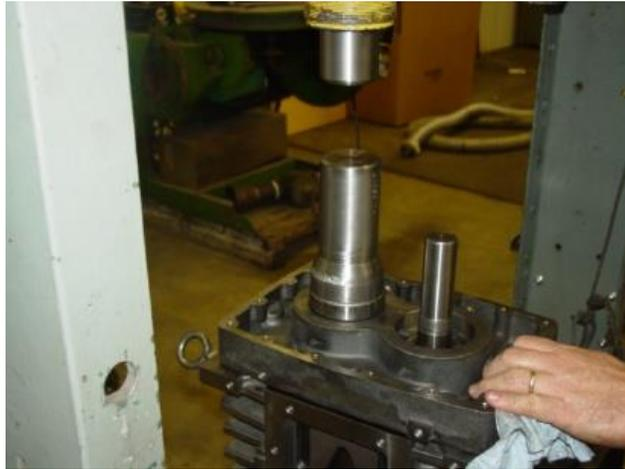
**FIGURE 8-3 – PRESS BEARING ONTO ROTOR SHAFT**
