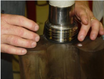
FIGURE 7-1 – INSTALL PISTON RINGS
