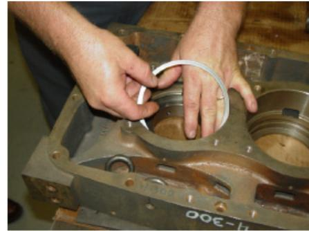
FIGURE 7-2 – INSTALL RETAINING RING
