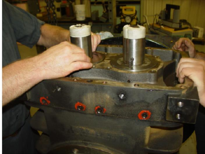
**FIGURE 7-8 – INSTALL FALSE BEARINGS IN BOTH BEARING BORES**
