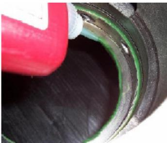
FIGURE 7-3 – LOCTITE 620 BEARING HOUSING
