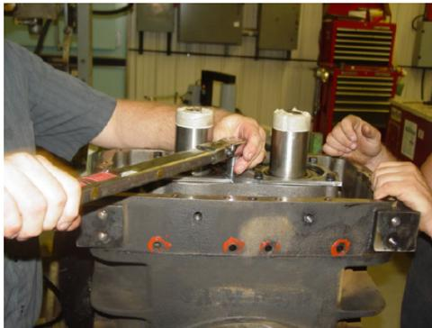
**FIGURE 7-10 – TORQUE THE SCREWS 38-41 FT. LBS.**
