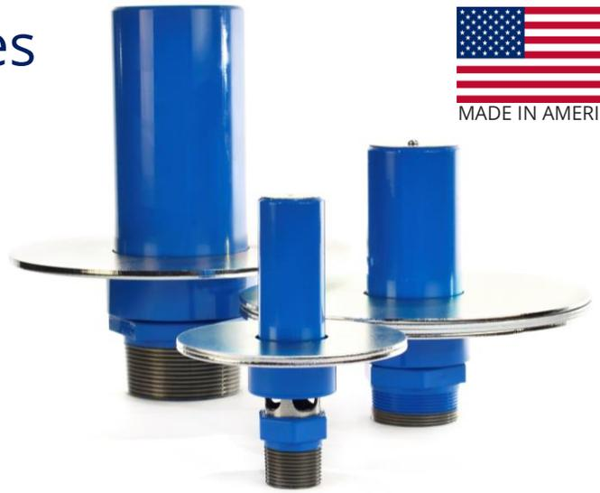
**INSTALLATION:** Relief valves must be mounted in the vertical position to assure proper operation. The relief valve is installed on the discharge side of the blower, before any valves, preferably immediately after a silencer if one is supplied
